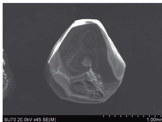
Figure 2. General appearance of the Capii-06 diamond under natural light (top) and in an SEM image. The figures show the slightly distorted rhombohedral shape of an intact crystal.
